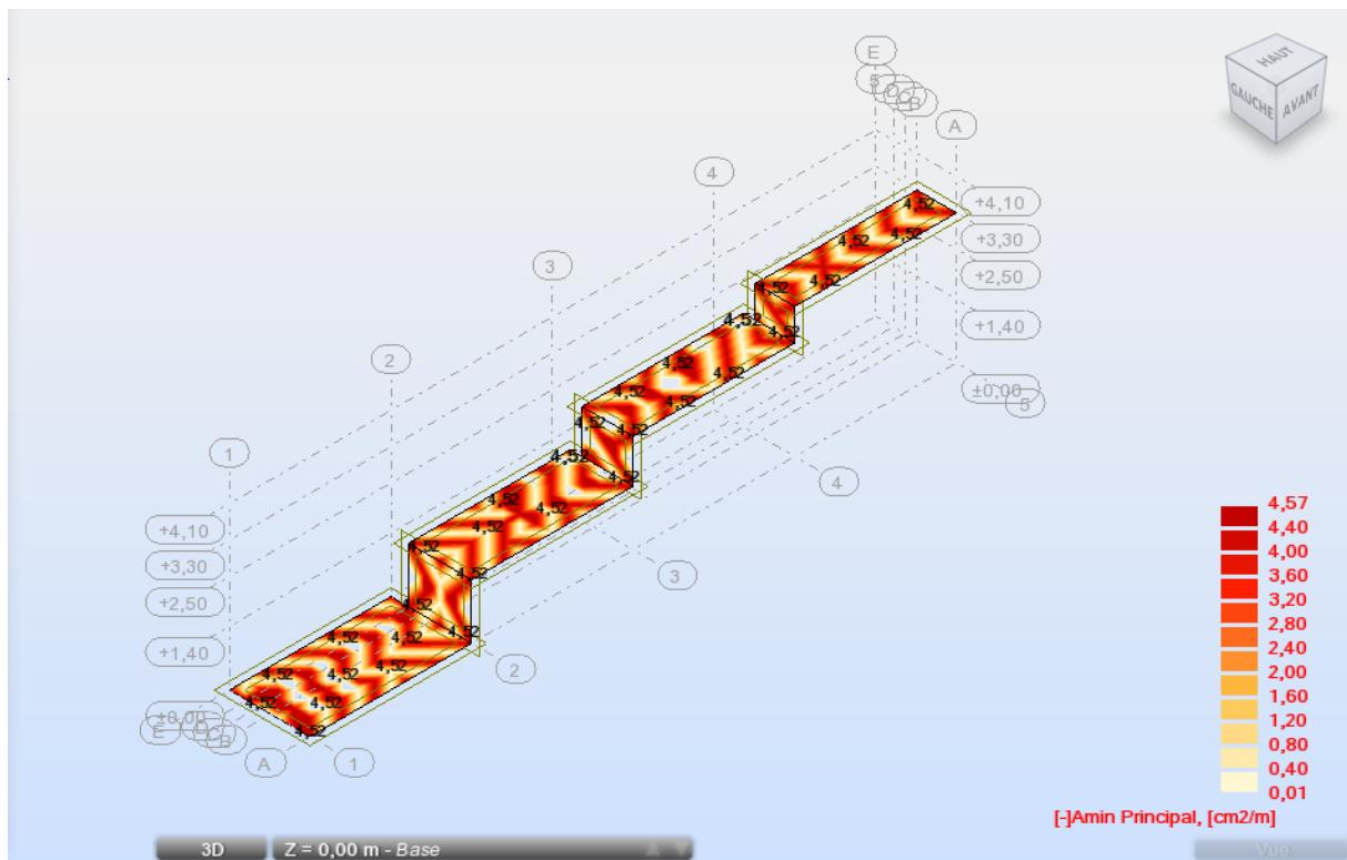
Figure 53: Armatures minimales
