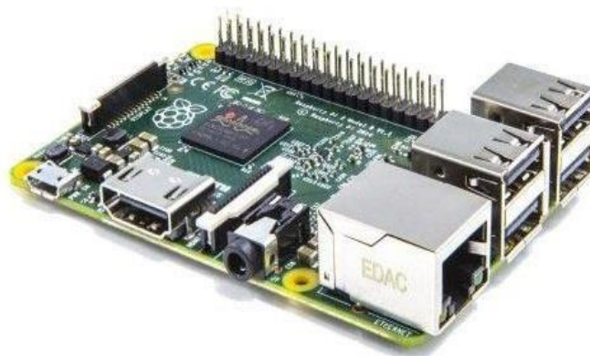
Figure II. 2 : Raspberry Pi Model B Source: @raspberrypi/Page Facebook
