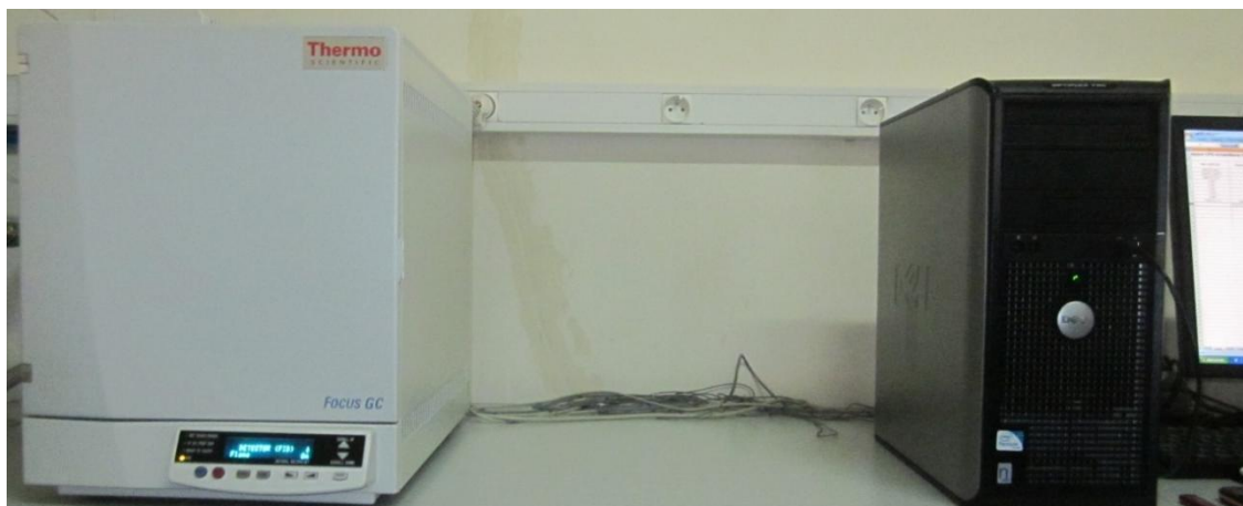
Figure 17: Chromatographe Focus GC (Cliché : Razafimamonjison, 2013)
